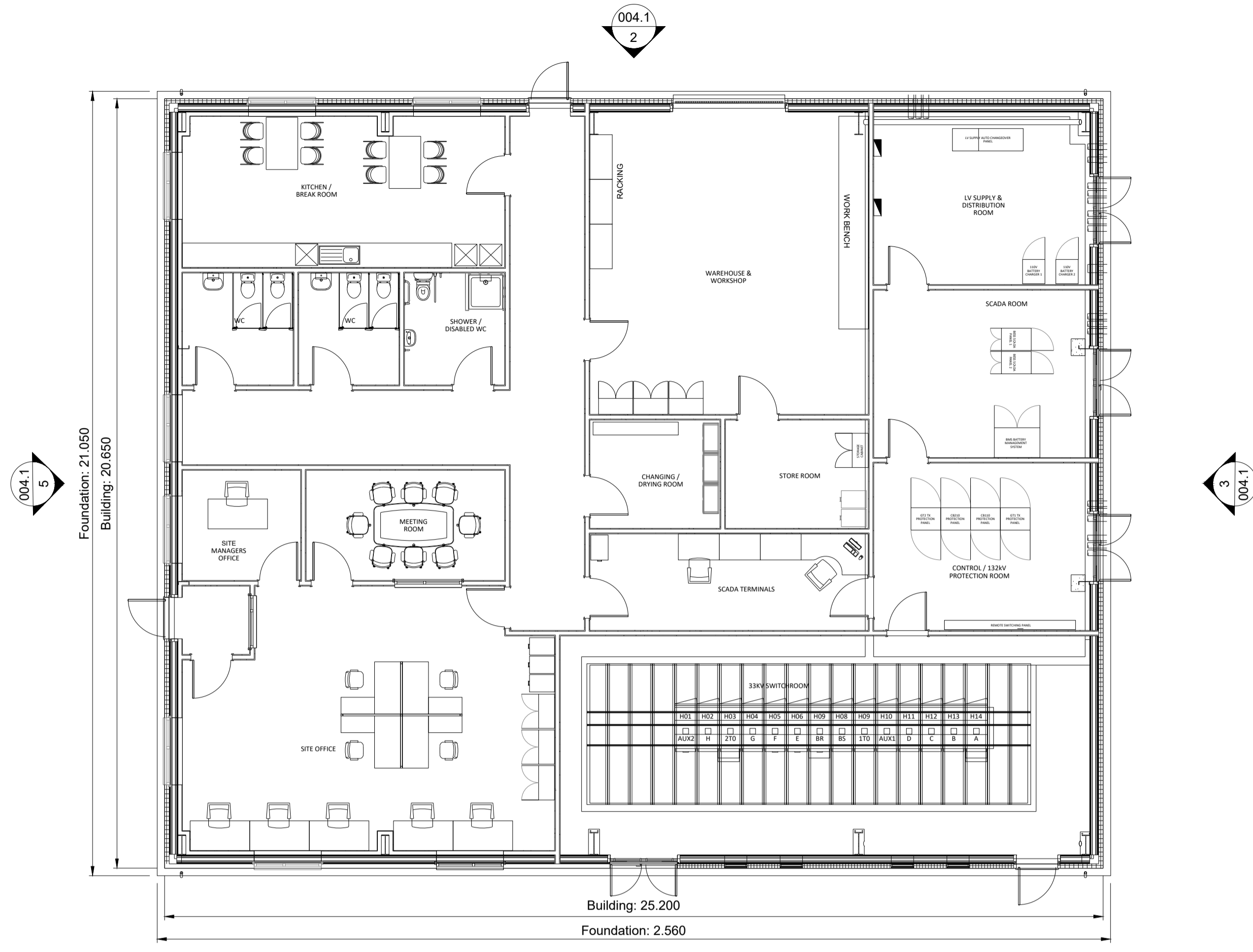
1 Substation Building Plan Scale 1:100 @ A1
